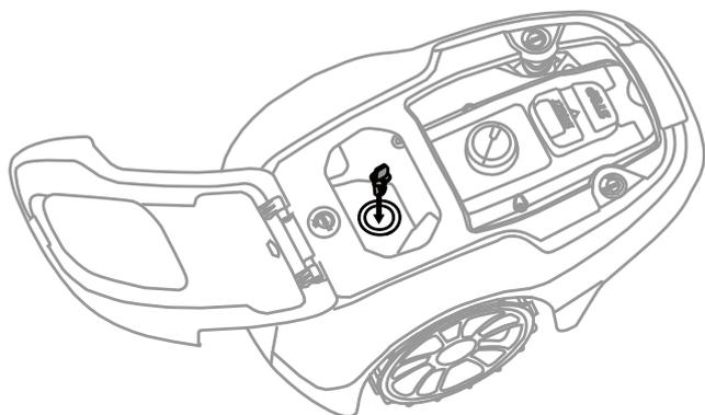
Insert the safety key into the mower and turn to the ON" ( I ) position.
