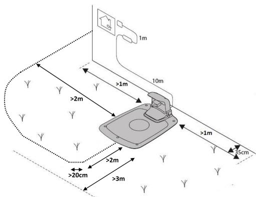
Run the guide wire to the loop on the boundary wire where the guide wire is to be connected.
