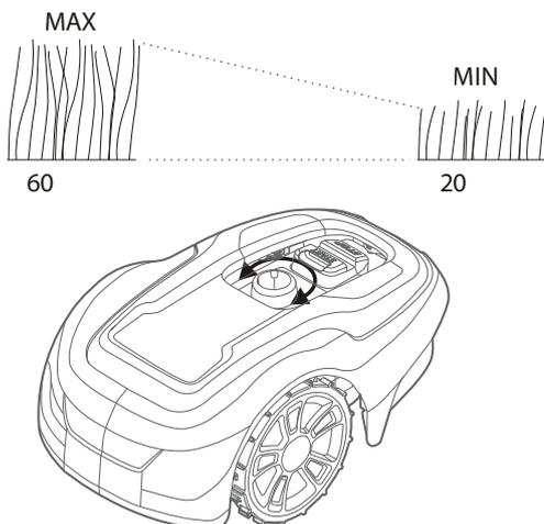
For the first few weeks of mowing, set the cutting height to 60 mm to avoid cutting the boundary wire and guide wire. Lower the setting one step each week thereafter until the desired cutting height is reached.
