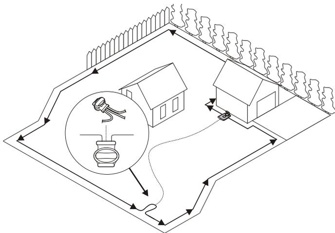
The mower uses the optional guide wire to find its way back to the charging station, but also find hard-to reach areas of the operating area. For example, the guide wire is laid between the charging station and a remote part of the working area or through a narrow passage.
