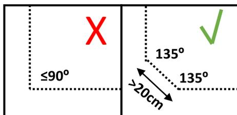
Do not lay the guide wire at sharp angles or the mower will have difficulty following it.
