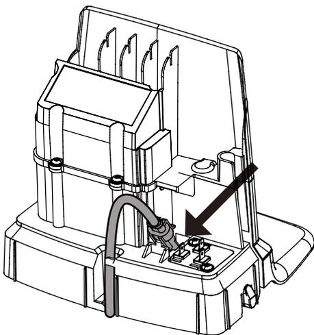
Connect the low voltage cable to the charging station.
