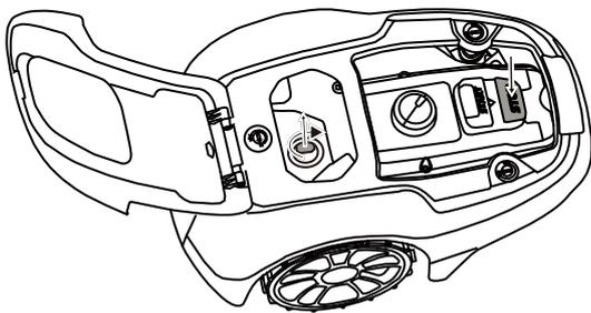
Press the **STOP** button on the mower and remove the safety key.
